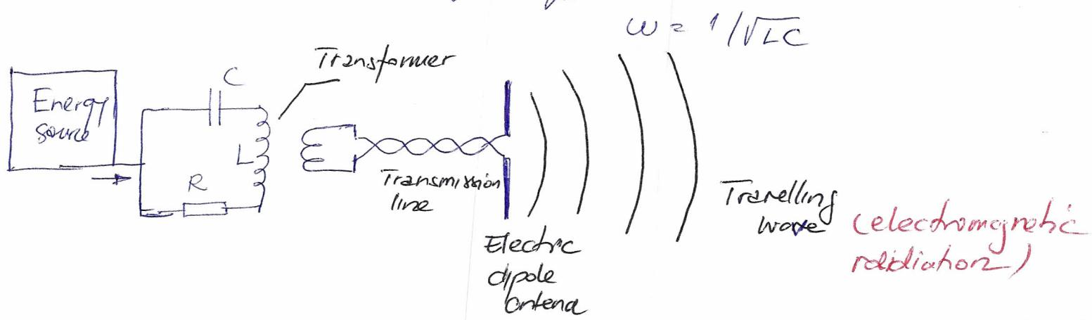
Antenna has the role of an electric dipole, being constituted of two thin conducting rods. The oscillatory current in the oscillator (RLC) causes charge to oscillate sinusoidally in the rods of antenna at the angular frequency  $\omega = 1/\sqrt{LC}$ .  $\Rightarrow$  electric dipole moment varying sinusoidally in time  $\Rightarrow \vec{E}(t) \rightarrow \vec{B}(t) \dots$
